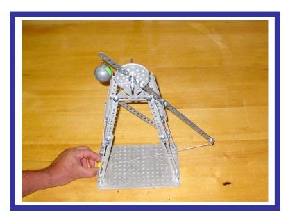
The projectile is a 5 gram (0.18 oz), 1" diameter wood ball with a total ball and sling length of 12" (305 mm).
