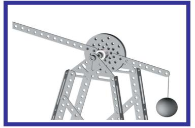
2.) The Counter weight is allowed to hang freely from the throwing arm as shown in the illustration above.
