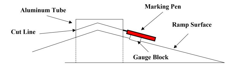
• The aluminum cylinder is perpendicular to the surface of the playing field. The intersection of the aluminum cylinder and the ramp does not form a circle, rather it forms an ellipse. An approximation of this elliptical intersection is shown below. The dimensions are spaced <sup>1</sup>/<sub>2</sub>" apart. Use these dimensions to create a paper pattern that can be transferred to the ramp. Use the paper pattern to trace a cut out for the intersection between the cylinder and the ramp.
