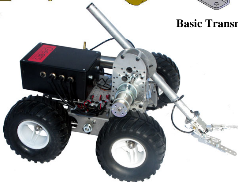
Transmission with Arm and Limit Switches Fitted to a Mobile Robot
