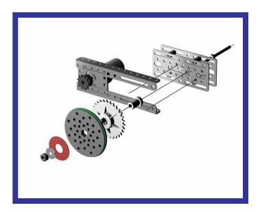
The Shaft Plates should be attached by threading four #10-24 machine screws through the 13 hole angles and into the four #10 standoffs. This is similar to how the motor and motor mounts are attached. The shaft plates can be attached anywhere along the length of the angle. This allows the length, and configuration of the chassis to be adjusted as needed.
