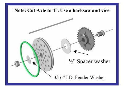
Leave the setscrews loose until the final assembly. Do not over tighten the setscrews.
