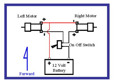
Note: These motors are fixed magnet DC motors. Right and left side motors turn in opposite directions. The direction of a fixed magnet DC motor is determined by the polarity, or direction of the current through the motor.
